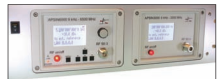
▲ Fig. 5 Nineteen-inch rack mount holding two APSIN signal generators at 3U height and 30 cm depth.
