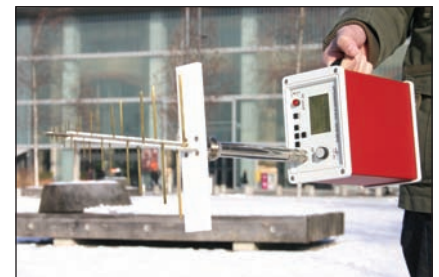
▲ Fig. 4 The mains-free operation provides advantages in field testing.
